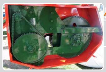
A chain and gear transmission reduces hydraulic motor rpm and generates the torque to handily discharge up to 200 bushels of grain per minute.
