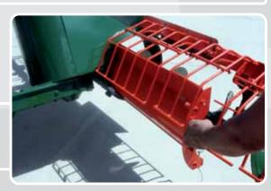
A sliding partition seals the reception chamber and speeds up the passage of grain through the auxiliary hopper.
