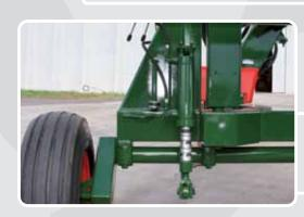
Height regulation for transport and work is set hydraulically and cylinder clamps are used to ensure steadiness in operation.
