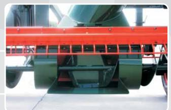
The amount of incoming grain is boosted by a patent pending reception chamber that includes new scooped pusher vanes for unmatched delivery of grain to the discharge auger.
