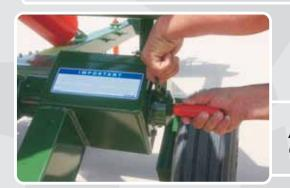
A simple pull-type locking mechanism connects and disconnects the sweeper augers in a snap.
