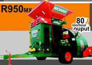
With 80 metric tons (3,150 bushels) per hour output, the R950MX is the largest 9 ft. crimper-bagger in the business. A 300 ft. long bag can hold 320 metric tons (12,600 bushels) of produce.
